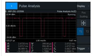
All R&S®NRP-Z8x wideband power sensors allow automatic pulse analysis. Up to 12 of 18 user-selected pulse parameters can be displayed in addition to the measurement trace.
